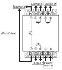
Note: 1. The Time Switch output uses a no-voltage contact. An external power supply is required for applications in which a load is driven.
